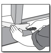
[2] Undercut doorjambs for a professional fit. Doorways less than 6' wide require T-Molding.
